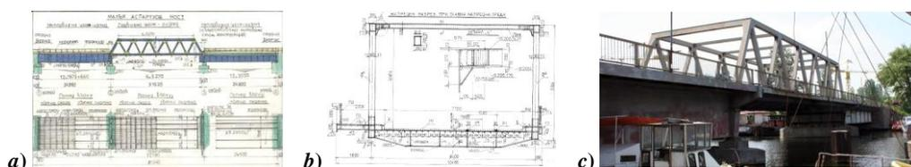
Figure 7a,b,c. “Varna Lake” movable bridge: Longitudinal section-a), Cross-section-b), View of the orthotropic bridge-c)
