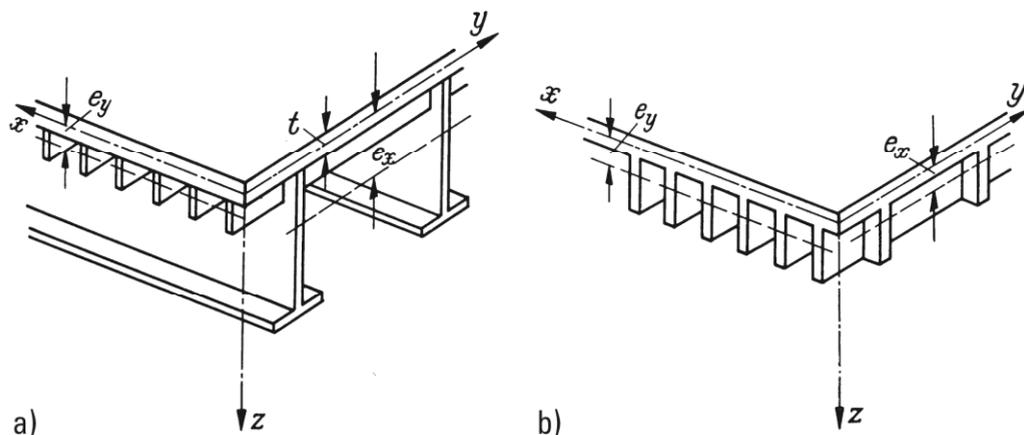
Figure 4a,b. Plate cross-sections around 1960; flat steel plate (bridge-building)-a), integral plate (aircraft construction)-b)
