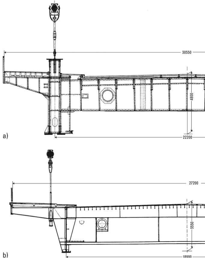
**Figure 3a,b. Mülheim suspension road bridge over the river Rhine, of supporting distances 85,0 + 315,0 + 85,0 m; Sections: old-a) and new bridge-b)**
