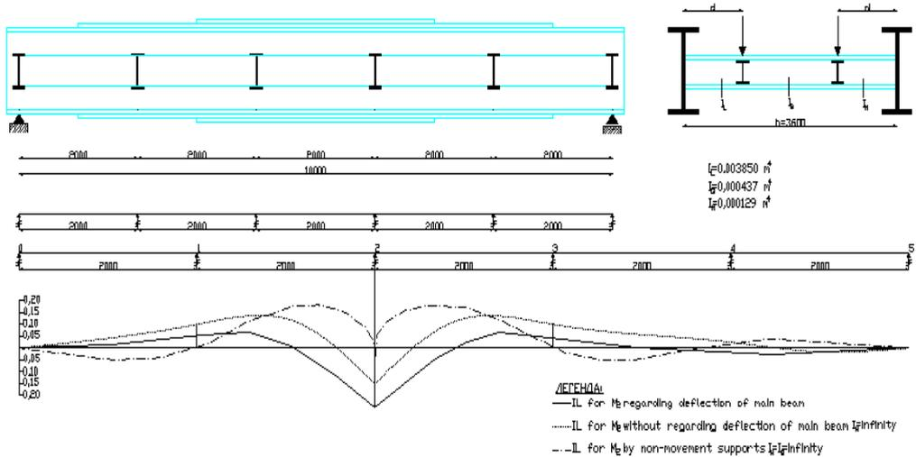
Figure 2. Railway bridge of 10-meter span. Comparing influence line for a bending moment in longitudinal beam in point 2
