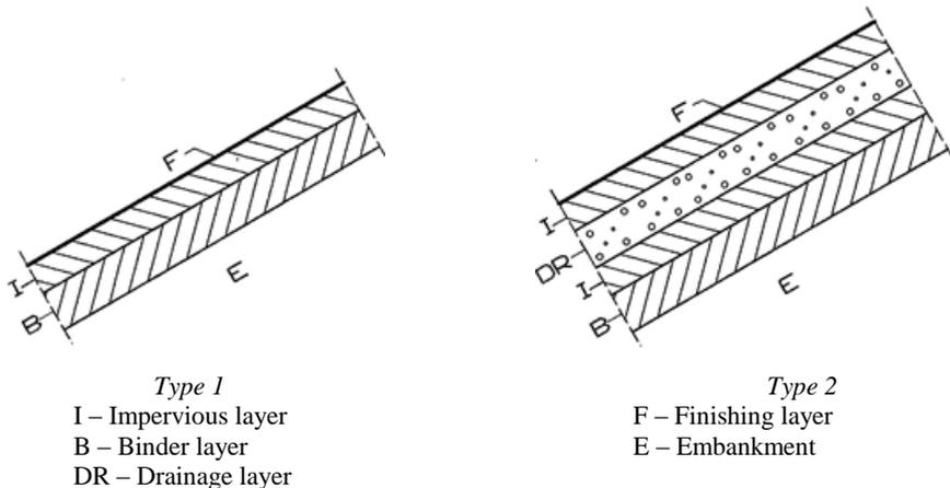
**Fig. 1. Basic Systems of Asphalt Concrete Linings**
