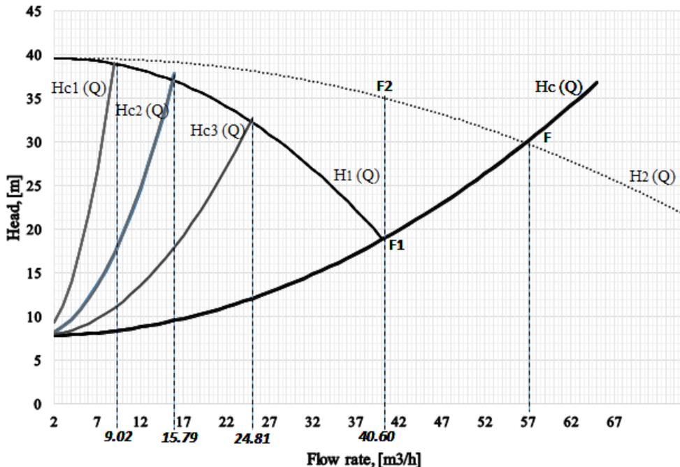
Figure 2. Constant speed pumps. Main operation points
