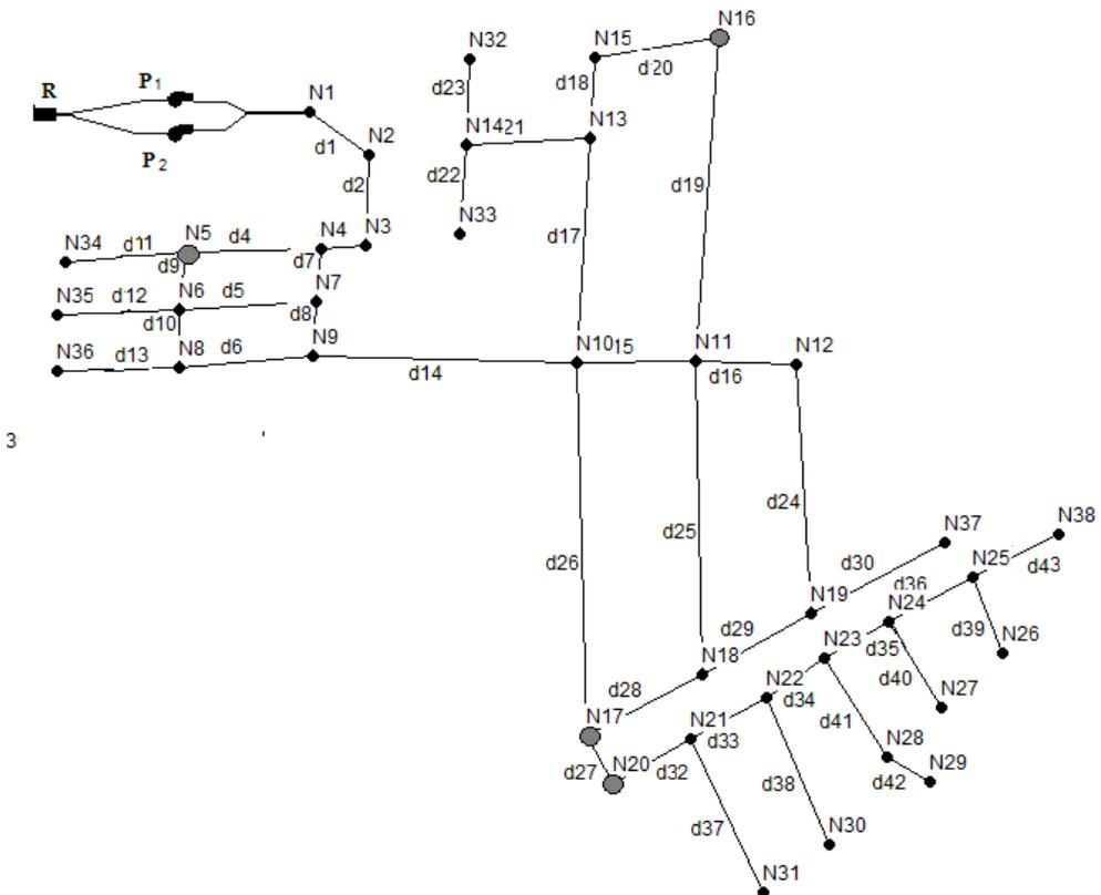
Figure 1. Tariverde water distribution system. Grey circular marker for the nodes with extreme elevation values
