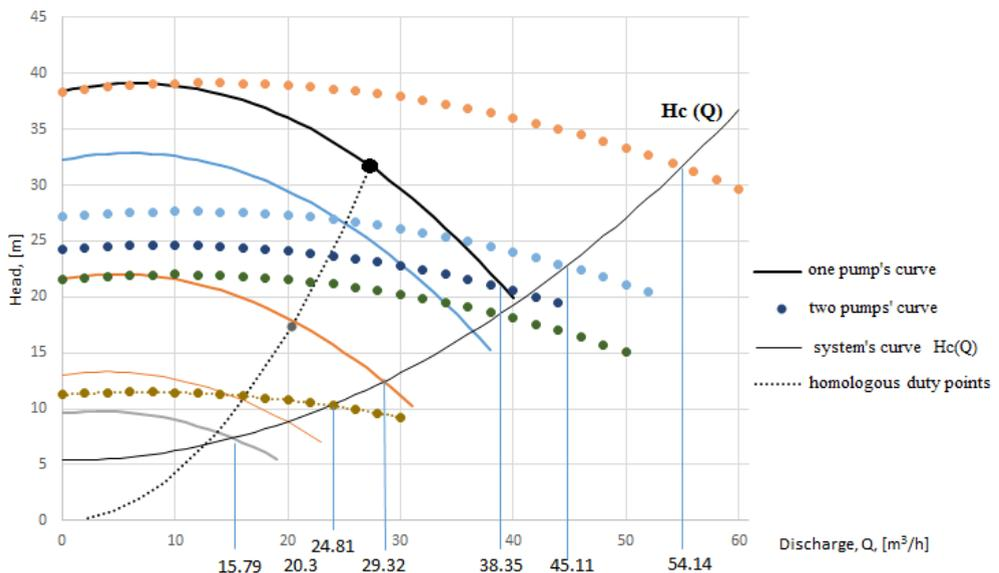
Figure 3. Variable speed pumps. Operation points
