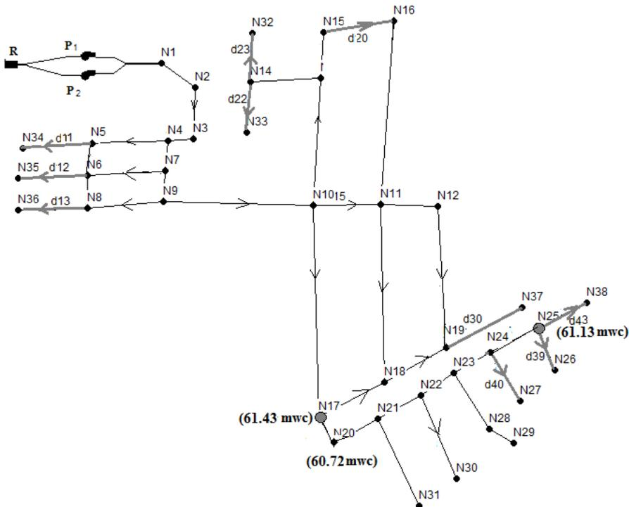
Figure 4. Constant speed pumps. Maximal pressure values at 4 a.m., expressed in mwc (meter water column)
