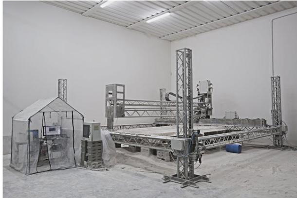
Figure 5. Concrete printing Printer [www.3DPrint.com]
