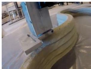
Figure 2. 3D Concrete printer in operation [12]
