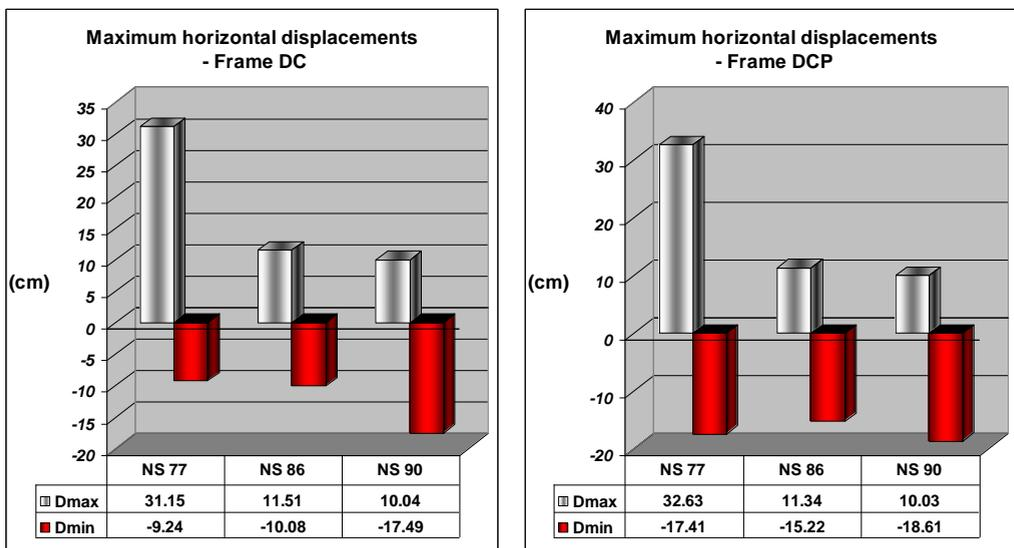
Figure 3. Extreme values of the lateral roof displacements noticed for frame DC and frame DCP
