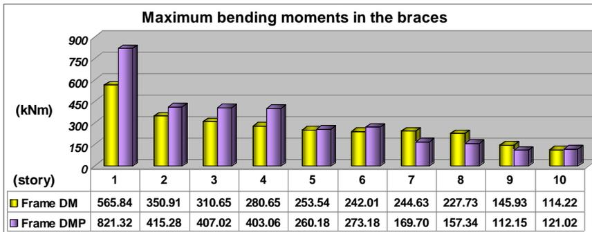
**Figure 9. Maximum bending moments in the braces of frame DM and DMP**
