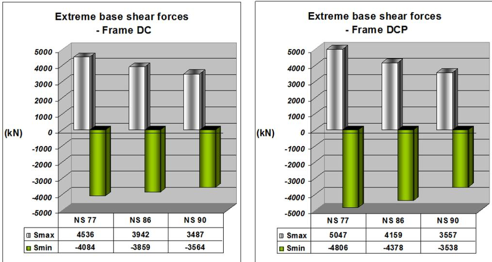
Figure 2. Extreme values of the base shear forces recorded for frame DC and frame DCP
