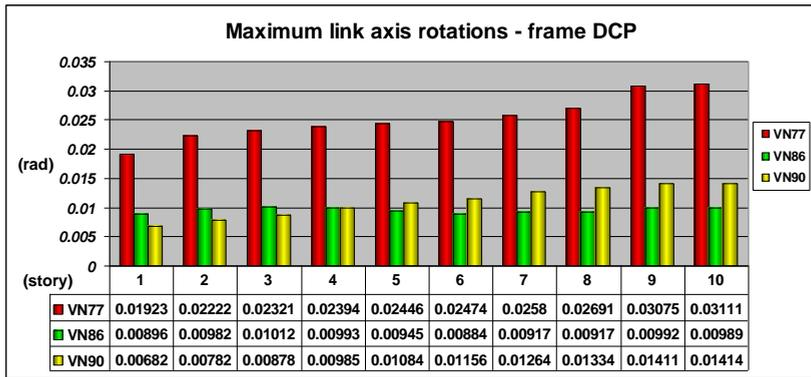
Figure 6. Maximum plastic deformations in the dissipative members of frame DCP
