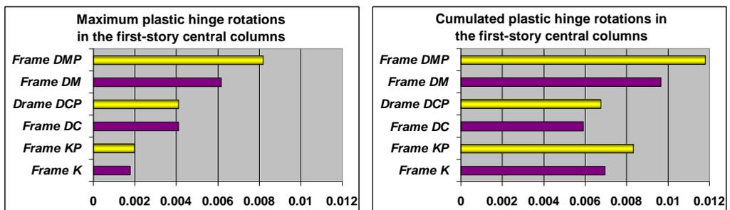
Figure 12. Maximum plastic deformations recorded in the bottom-storey central columns
