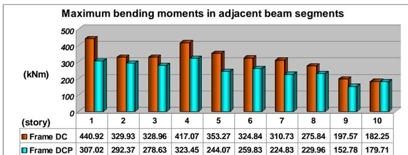
Figure 8. Maximum bending moments in the adjacent beam segments of frame DC and DCP
