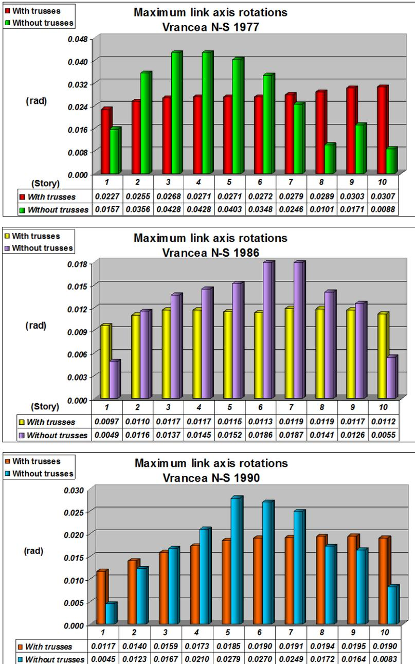
Figure 4. Maximum plastic deformations in the dissipative members of frame K and KP
