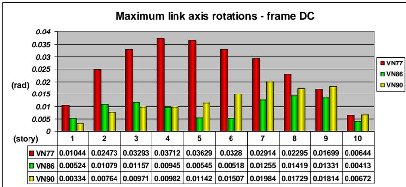
**Figure 5. Maximum plastic deformations in the dissipative members of frame DC**
