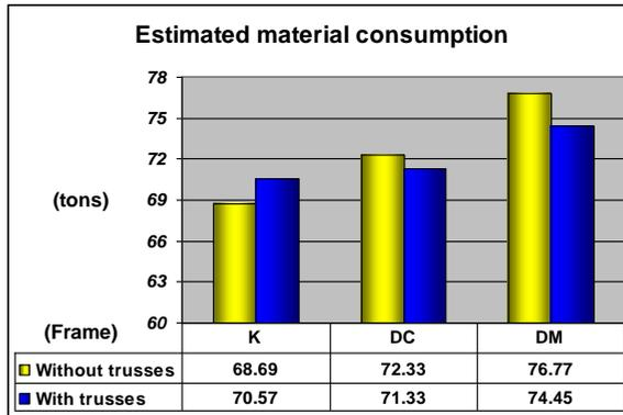
Figure 13. Estimated material consumption for the six analyzed frames
