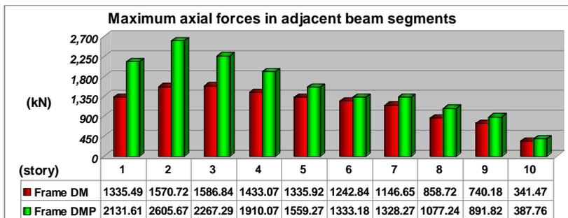
Figure 7. Maximum axial forces in the adjacent beam segments of frame DM and DMP
