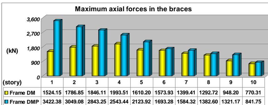
**Figure 10. Maximum axial forces in the diagonals of frame DM and DMP**
