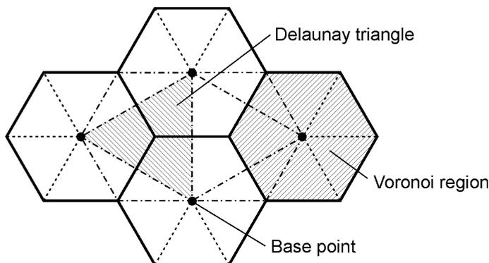
Figure 2. Top view of the mesh layout of the RSim-3D model with polyhedral cells [18]
