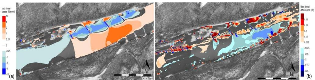
**Figure 6. (a) Bed shear stress differences, (b) difference of differences of bed level changes, between increased crest elevation and reference condition for MQ [23]**
