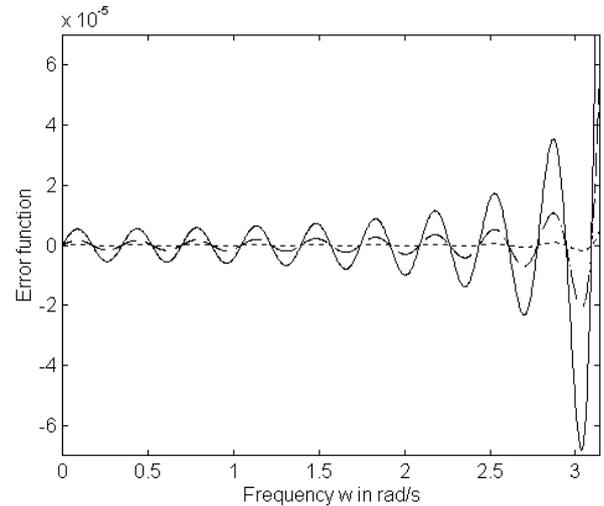
Fig.3. The error curves for fullband differentiators ( $N=36$ ) with three different orders  $k$  ( $k=9$  – solid line,  $k=11$  – dashed line,  $k=15$  – dotted line).
