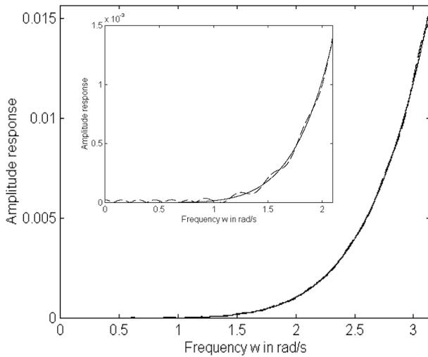
Fig.1. An ideal (solid line) and designed (dash dot line) amplitude responses.
