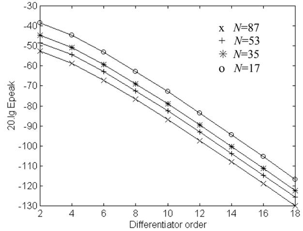
Fig.2. Variation of  $20\log_{10}E_{\text{peak}}$  with differentiator order for four different values of filter length  $N$ .
