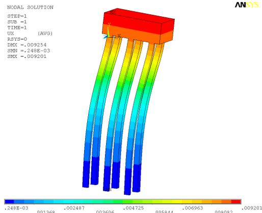
Figure 5. Displacements of the pile frame (isolated), ANSYS
