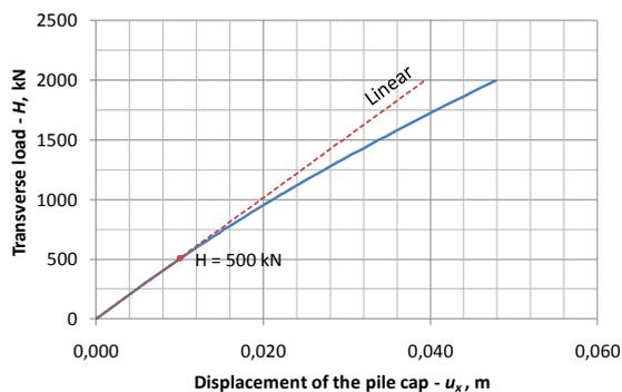
Figure 7. Load-displacement curve from PLAXIS 3D
