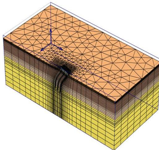
Figure 6. Computational model in PLAXIS 3D Foundation
