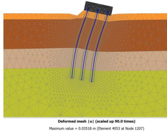
Figure 3. Deformed mesh around the frame, PLAXIS 2D
