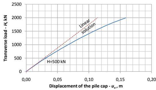
Figure 4. Load-displacement curve, PLAXIS 2D
