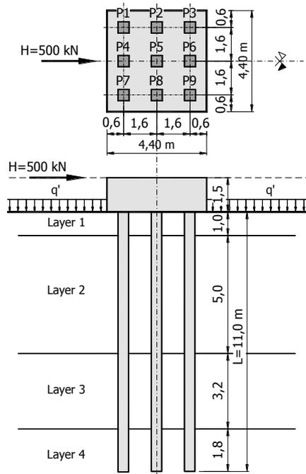
Figure 1. Pile frame geometry and soil layers
