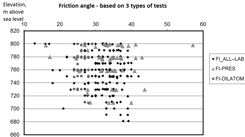
Fig. 3 Friction angle \phi ( ^{\circ} ) for the tailings dam material – laboratory tests, pressuremeter, dilatometer
