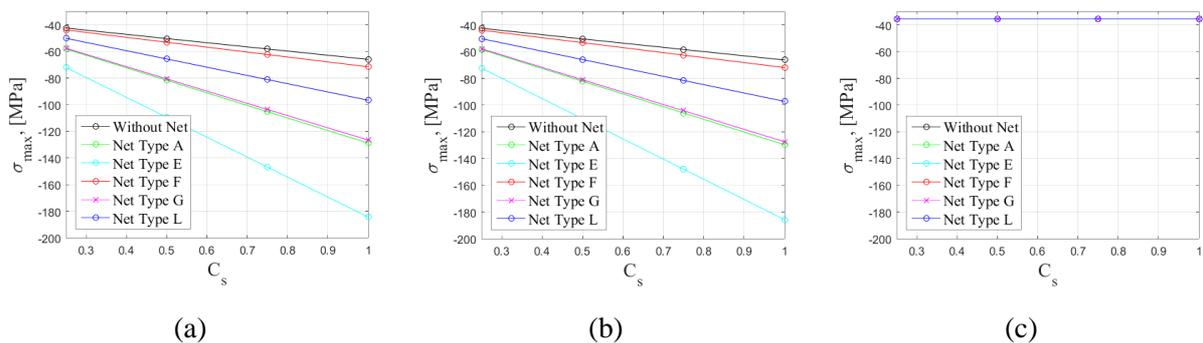
Figure 6. Maximum normal stress (compression) in most loaded standards in load combination a) Service condition: (a) Scheme 1, (b) Scheme 2, (c) Scheme 3.
