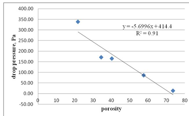
**Figure 3.** Relationship between porosity and pressure drop on nets at wind speed 26,1 m/s.
