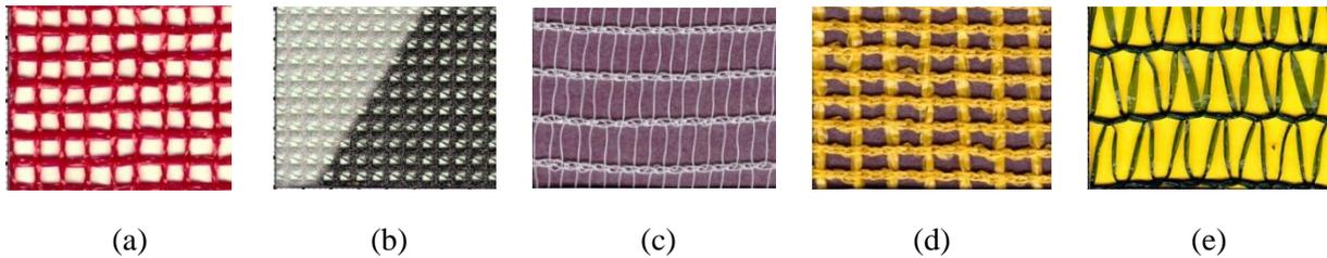
**Figure 2.** Samples of nets: (a) net type “A”, (b) net type “E”, (c) net type “F”, (d) net type “G”, (e) net type “L”. Images are indicative and not to scale.
