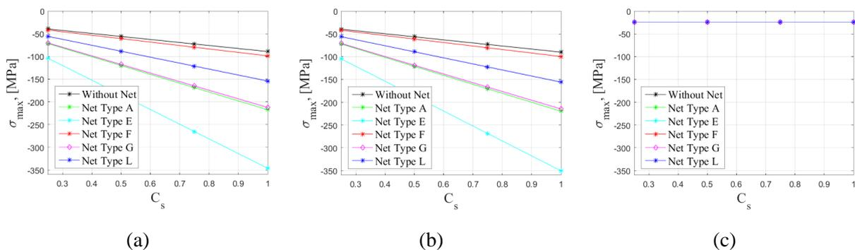
Figure 7. Maximum normal stress (compression) in most loaded standards in load combination b) Out of service condition: (a) Scheme 1, (b) Scheme 2, (c) Scheme 3.
