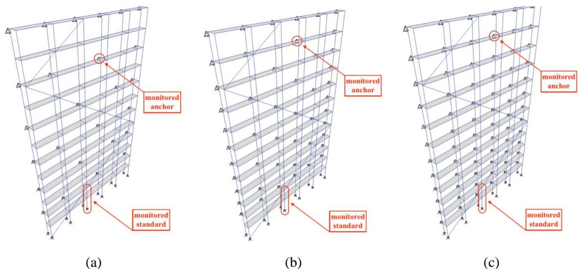
**Figure 1.** Static scheme of the scaffolds: (a) Scheme 1, (b) Scheme 2, (c) Scheme 3.
