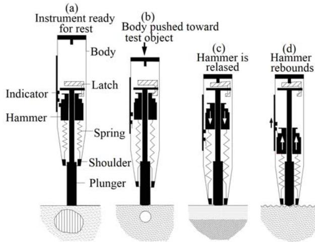
FIGURE 3. Principle of the rebound hammer test [12].
