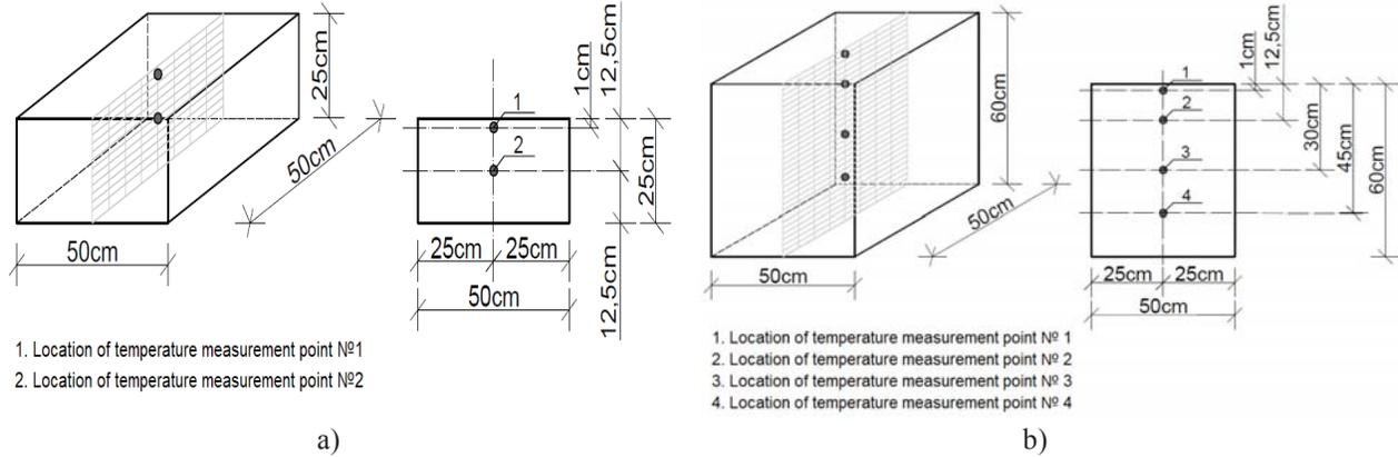
**FIGURE 2.** Locations of temperature measurement points
