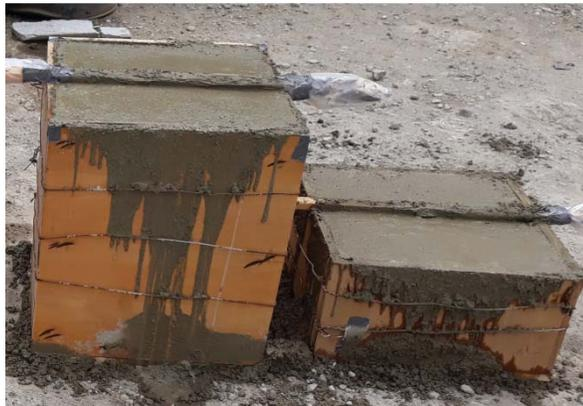
FIGURE 1. Test specimens after placing of the concrete.
