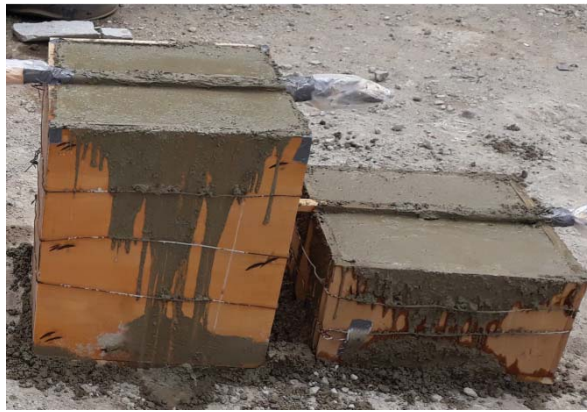
FIGURE 1. Test specimens after placing of the concrete.
