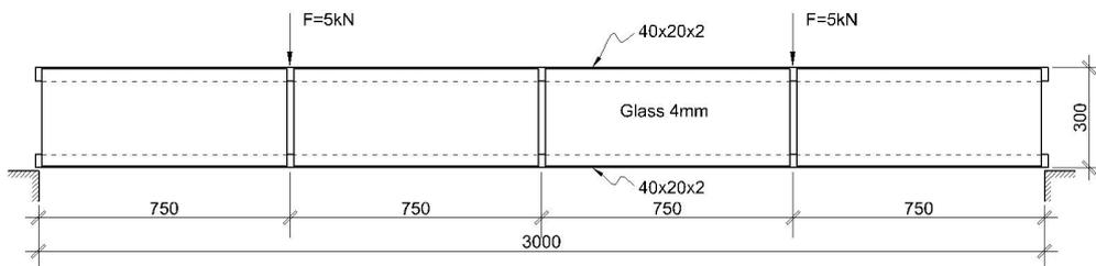
Figure 7. Schematic representation of the member analyzed.
