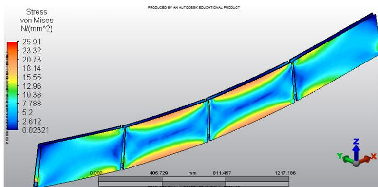
Figure 8. Stress von Mises diagram of the glass webs.
