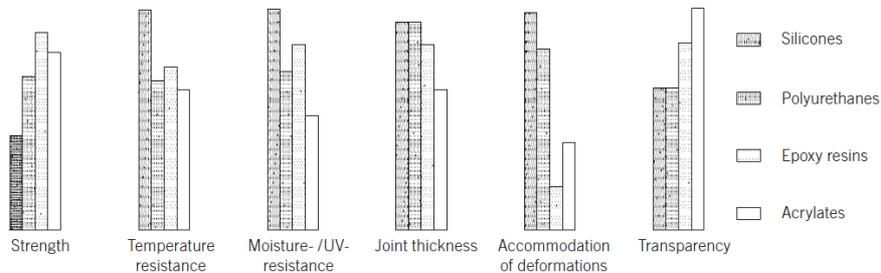
Figure 6. Properties of different types of adhesives, as in [4].
