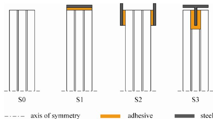
**Figure 1.** Half cross sections of tested beams, as in [3]. Laminated glass beam without reinforcement tested for comparison.
