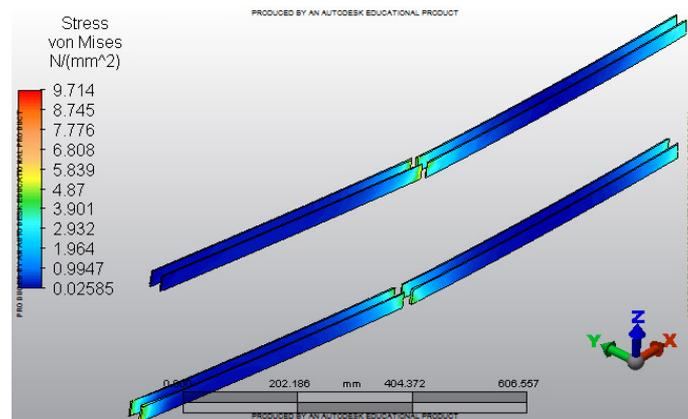
**Figure 9.** Stress von Mises diagram of the adhesive.
