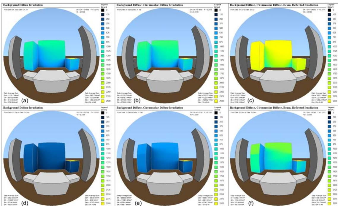
**Fig. 4** Exemplary images, generated in 3D–SOLARIA Irradiation Mode – average daily irradiation under a real sky in Sofia: (a) background diffuse irradiation in July; (b) diffuse irradiation in July; (c) diffuse, beam and reflected irradiation in July; (d) background diffuse irradiation in December; (e) diffuse irradiation in December; (f) diffuse, beam and reflected irradiation in December
