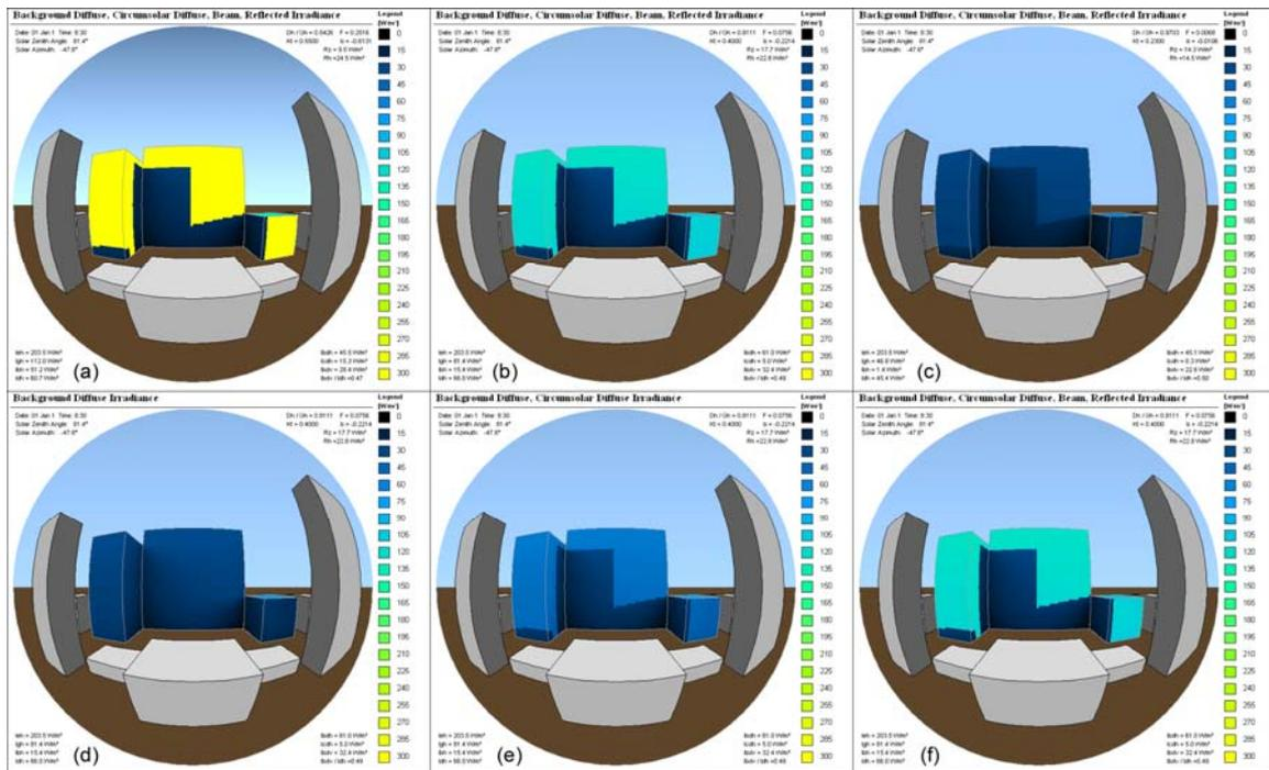
**Fig. 3** Exemplary images, generated in 3D-SOLARIA Irradiance Mode for January 1<sup>st</sup>, 8:30 in Sofia: (a) solar irradiance –  $D/G=0.54$ ,  $K_t=0.55$ ; (b) solar irradiance –  $D/G=0.81$ ,  $K_t=0.4$ ; (c) solar irradiance –  $D/G=0.97$ ,  $K_t=0.23$ ; (d) background diffuse irradiance –  $D/G=0.81$ ; (e) diffuse irradiance –  $D/G=0.81$ ; (f) diffuse, beam and reflected irradiance –  $D/G=0.81$
