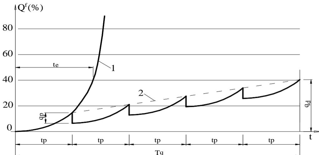
fig. 2 Scheme for determination of the period of the use  $T_q$  the period between repairing works  $t_p$
