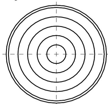
fig. 4 Location of ring shaped stiffening girders under the membrane
