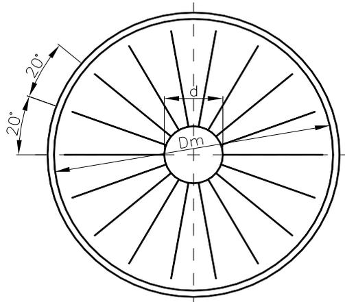
fig. 10 Membrane stiffened with radial located girders and central pontoon
