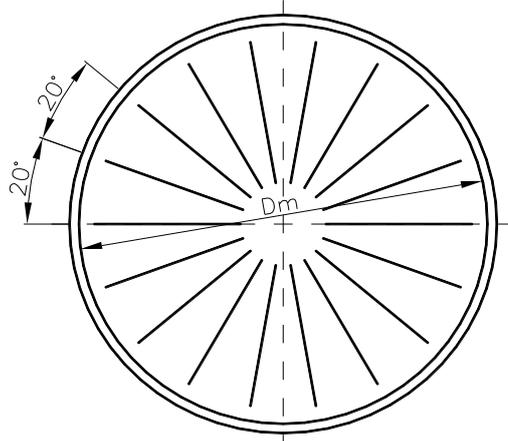
fig. 8 Membrane stiffening with radial girders
