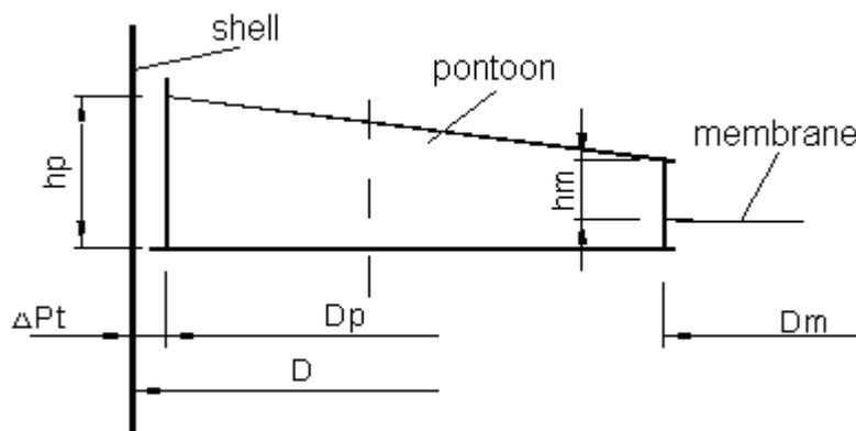
fig. 2 Basic dimensions of shell and pontoon
